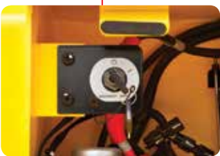
Master Switch A master switch disconnects the battery power to protect the electrical system from excess electrical drainage.
