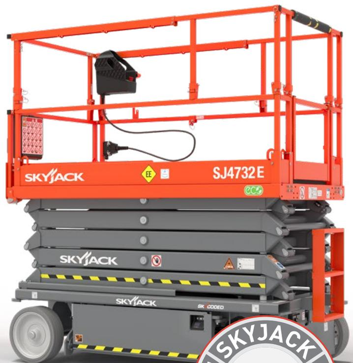
Classification: Skyjack scissor lifts equipped with “EE” Rating Package can be used in Class I, Division II, Group D locations as specified by the NFPA 505 Fire Safety Standard.
